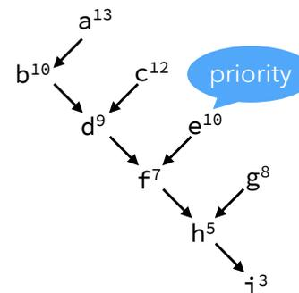
A node's priority is the length of the longest latency-weighted path from it to a root of the dependence graph
